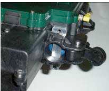
6 – B. For Red and Yellow cylinders leave the backing plate open and re-install the "T" Key
