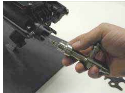
Then pull the barrel off. This will reveal the injection piston.
