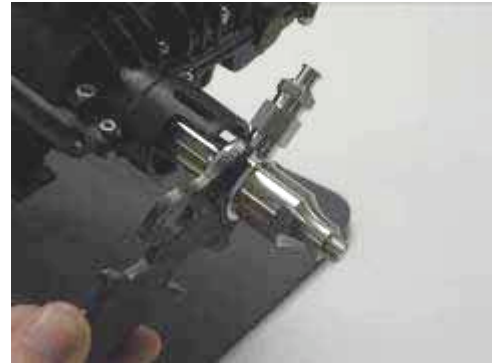
Using the wrench provided, loosen the barrel.
