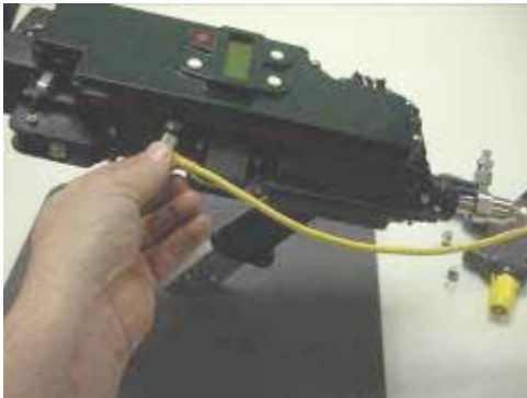
Locate the plug connection on the side of the injector and insert the yellow cable.
