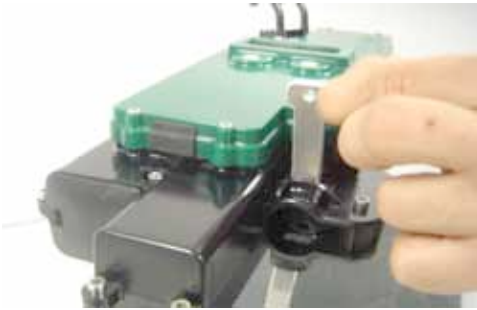
2. Remove cylinder "T" key
