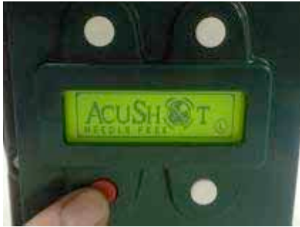
1. Press the RED button to start
