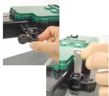
6-A. For Pink, Green & Blue cylinders. Swing the cylinder backing plate into original position and re-install the "T" key
