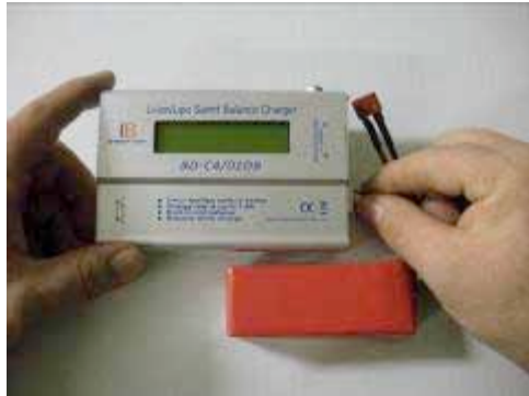
1. Plug battery into the battery charger
