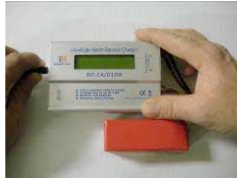
2. Plug the power adapter into the battery charger
