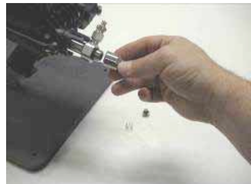
Reinstall the barrel nut ONLY . WITHOUT THE VALVE AND SPRING and tighten the barrel nut.
