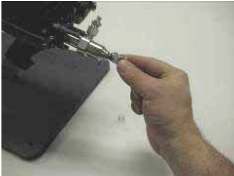
Install extension adapter and tighten
