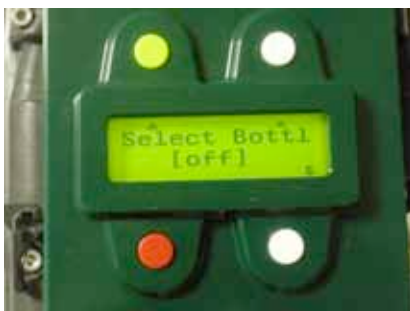
5. Select the supply container size (#6)
