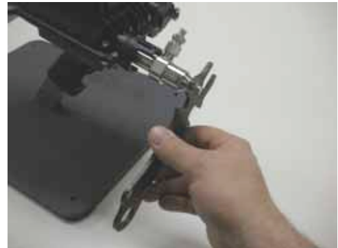
Using the wrench provided, unscrew orifice and remove it completely.
