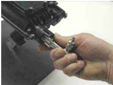
Turn the barrel until you reach the end of the thread.
