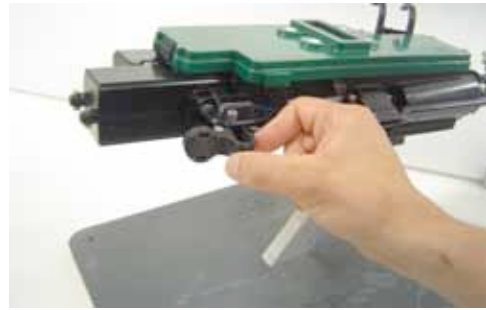
3. Pull out and swing away cylinder backing plate
