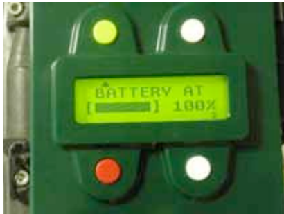
3. Verify battery condition (#2)
