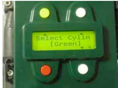
4. Confirm power cylinder selection (#4)
